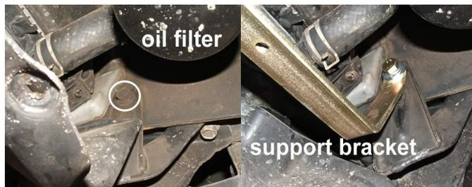
There are 3 extra M12 washers included. These may be needed to go between the front bracket and the chassis rail, to help lineup the holes on the bracket with the 3 x M10 bolts on the front plate for series 2/3's.
